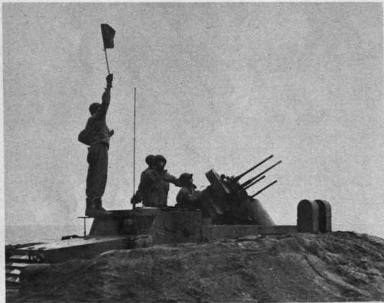
M-16's gun mount has four .50-caliber machine guns, giving it higher rate of fire than obsolescent M-13. Unlike the M-15, the M-16 has no revolving bucket. The turret mechanism is in a heavy, conical mount.
